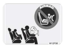
Never place a Child seat (Rear-facing or Front facing) restraint in front passengers seat, if passenger airbag is present. Because, If the airbag deploys could cause serious or Fatal injuries to the child.
