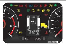
On inclines or curves, due to the movement of fuel in the tank, the fuel level may fluctuate or the low fuel level warning lamp may illuminate earlier than usual. Always check the fuel level when the vehicle is on level road.
