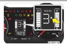
Higher gear position is selected for the vehicle speed or engine revolution. Changing to a lower gear position is recommended.
