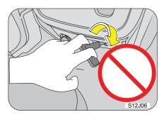
Do not attempt to release the Parking brake lever from top side. This may result in fingers get jammed with center console.
