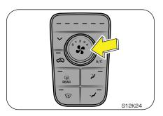
The blower force-circulates air through the HVAC unit and distributes it throughout the passenger compartment.
