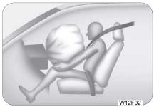
Front airbags are not intended to deploy in side-impact, rear impact or rollover crashes. In addition, front airbags will not deploy in frontal crashes which are below the prescribed deployment threshold where risk of serious injuries is low.
