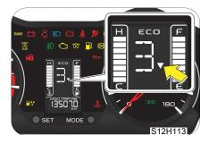
The control system monitors driving condition and it shows which gear position is optimal for driving with the indication on the display.
