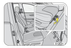
Move the seat forward or backward by lifting the adjustment lever located under the seat front and release once the desired position is reached.
