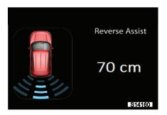
• If the obstacle is less than 50 cm, all bars in that direction will be turned ON and a STOP! symbol will be displayed
