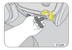
To release, Pull and Turn the Lever Clockwise and push it all the way forward.
