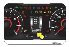
The bottom row of the LCD display gives the odometer reading. It records and displays the total distance traveled in kms.
