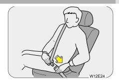
Adjust the seat as needed and sit up straight and well back in the seat. To fasten your seat belt, pull the webbing out of the retractor and insert the metal tab into the buckle. There will be an audible "click" when the tab locks into the buckle. Pull up on the shoulder strap to tighten the lap belt across your hips. The seat belt retractor will pull in any slack in the shoulder strap. A slow and easy motion will allow the belt to extend and let you move your body around freely.
