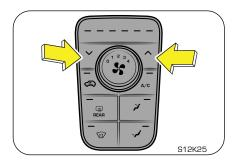
By operating the temperature control switch, temperature of air being discharged from various vents can be adjusted to the desired level. Engine coolant is utilized to heat, whereas the air conditioner is used to cool the air inside the AC unit. Based upon selected temperature switch- Up/Down, the desired discharged air temperature can be obtained.
