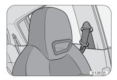
Your vehicle front seats are equipped with fixed head restraints. The head restraint help to avoid the whiplash injury on the neck in the event of rear collision.
